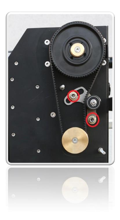
3. Tighten the belt like shown on the picture below (blue key). With the red key we tighten the screw.
