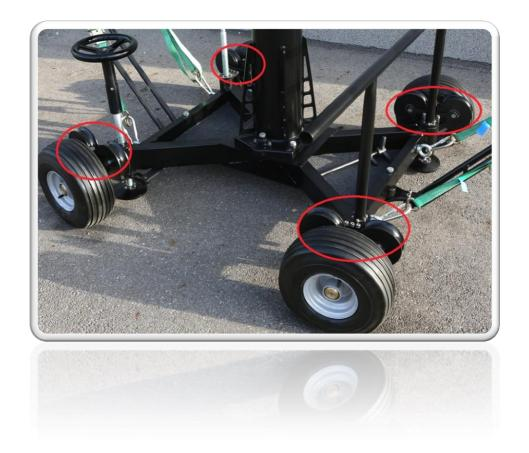
**D.3.** On the dolly there's a steering supported by 2 drawbacks connected to each other for best maneuvering of the crane. Optionally it's possible to block one of the drawback and separate it from the other one by dismounting the connecting strip under the dolly.
