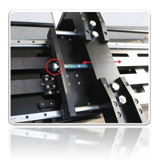
8. If the crane is still unbalanced after step 7, then we use donuts to balance it.
